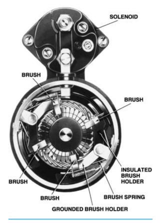
Figure 9-38. A four-brush motor. (Delphi Automotive Systems)
