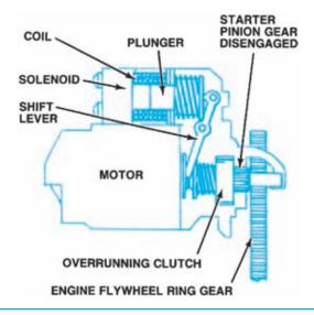
Figure 9-42. A typical solenoid-actuated drive.
