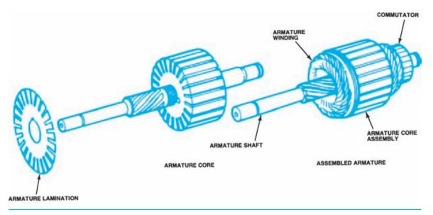
Figure 9-34. Motor armature.
