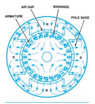
Figure 9-28. Flux path in a four-pole motor.
