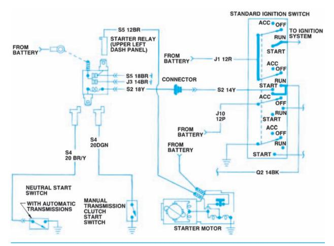
Figure 9-16. Typical DaimlerChrysler starting system. (DaimlerChrysler Corporation)
