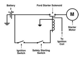
**Figure 9-15.** The Ford starting system circuit with the positive engagement starter.
