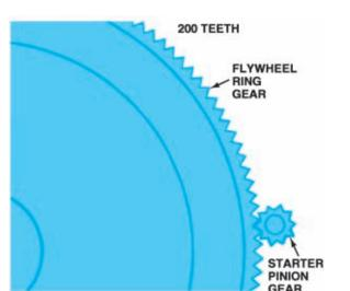
Figure 9-41. The ring-gear-to-pinion-gear ratio is about 20 to 1.
