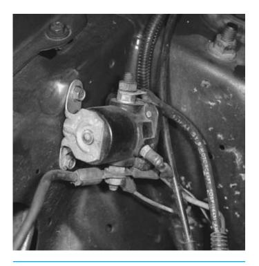
Figure 9-12. The Ford starter relay or magnetic switch.
