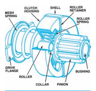
Figure 9-52. Cutaway view of an overrunning clutch.
