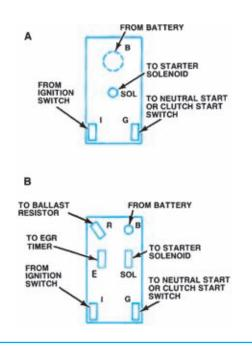
**Figure 9-17.** Comparison of the terminals on a pre-1977 starter relay (A) and a 1977 or later relay (B). (DaimlerChrysler Corporation)
