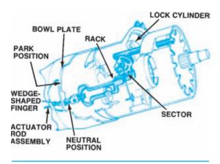
Figure 9-9. A mechanical device within the steering column blocks the movement of the ignition switch.
