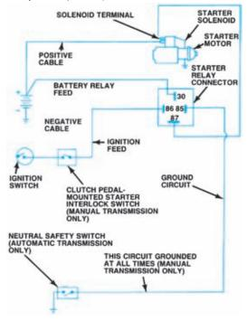
Figure 9-18. DaimlerChrysler starting system with a five-terminal relay. (DaimlerChrysler Corporation)
