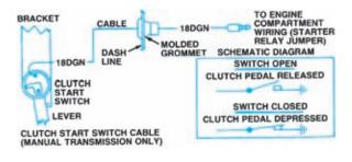
Figure 9-5. The clutch switch must be closed before battery current can flow from the magnetic switch to ground. (DaimlerChrysler Corporation)
