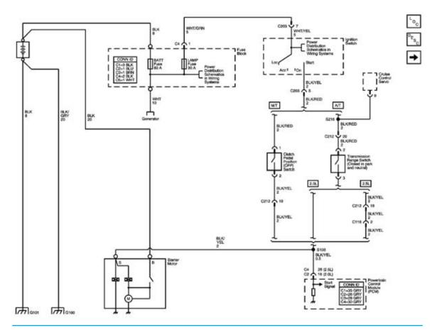
**Figure 9-4.** This starting safety switch must be closed before battery current can reach the magnetic switch. (GM Service and Parts Operations)
