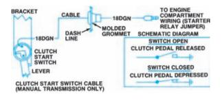
**Figure 9-20.** DaimlerChrysler clutch switch. (DaimlerChrysler Corporation)
