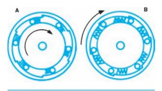
Figure 9-53. The operation of an overrunning clutch.
