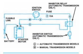
Figure 9-22. Typical Nissan starting system used on gasoline engines. (Courtesy of Nissan North America, Inc.)
