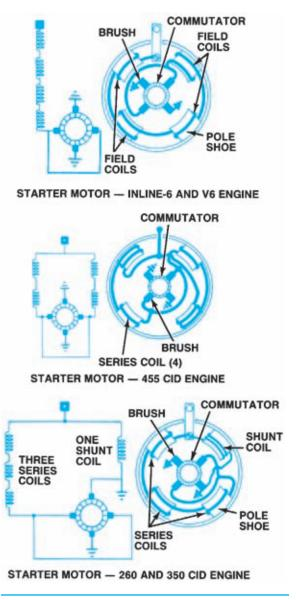
**Figure 9-46.** Delco-Remy provides differently connected starter motors for use with various engines. (GM Service and Parts Operations)
