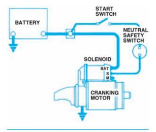
Figure 9-13. GM Starter circuit. (Delphi Automotive Systems)
