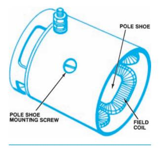
Figure 9-27. Pole shoes and field windings in housing.
