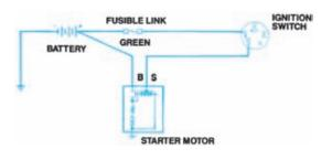
Figure 9-23. A typical Nissan diesel starting system. (Courtesy of Nissan North America, Inc.)
