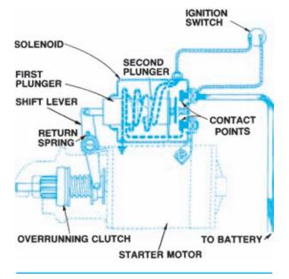
**Figure 9-47.** The Delco-Remy solenoid plunger is in two pieces. (Delphi Automotive Systems)
