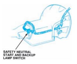
Figure 9-8. Transmission-mounted safety switch. (DaimlerChrysler Corporation)
