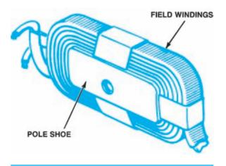
Figure 9-29. Pole shoe and field winding removed from housing.
