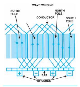
Figure 9-36. Armature wave winding
