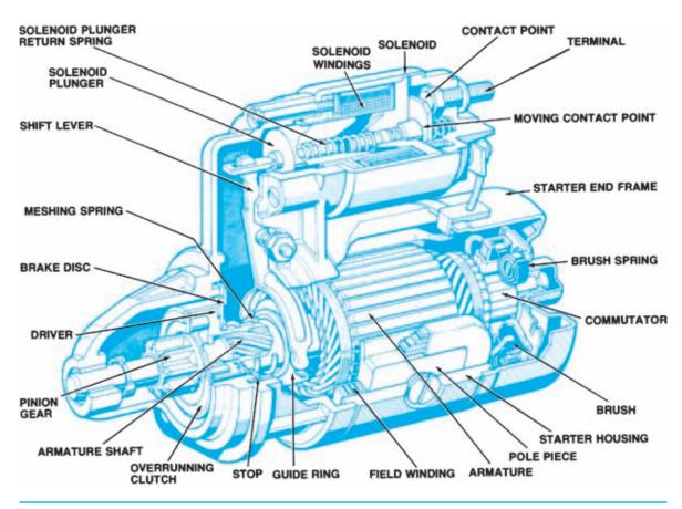
Figure 9-39. Starter motor cutaway.
