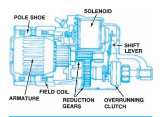
Figure 9-40. The Chrysler reduction-gear starter motor. (DaimlerChrysler Corporation)
