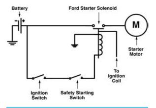
Figure 9-48. Circuit diagram of a system using a movable-pole-shoe starter.
