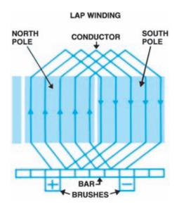
Figure 9-35. Armature lap winding. (Delphi Automotive Systems)
