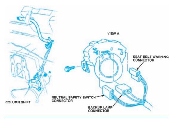
Figure 9-7. Column-mounted neutral safety switch near gearshift tube. (GM Service and Parts Operations)
