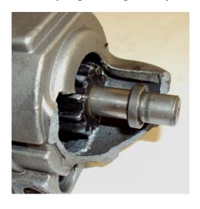
The problem is typically caused by an engine backfire or "kickback". GM has released Tech Service Bulletins addressing this issue; the cause is usually one of the following:
