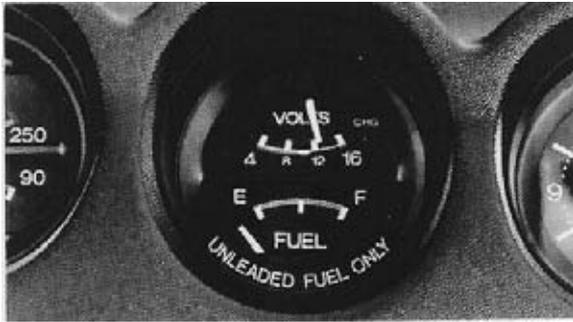
Figure 8-52. Automotive voltmeter in instrument panel.
