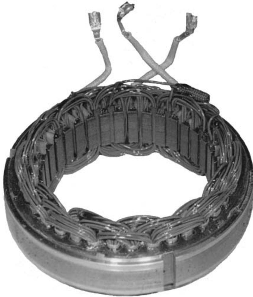
**Figure 8-14.** An AC generator (alternator) stator.
